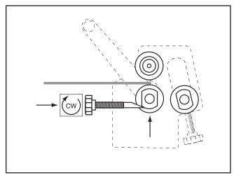
Figure 14. Raising bottom roller for flat rolling.
